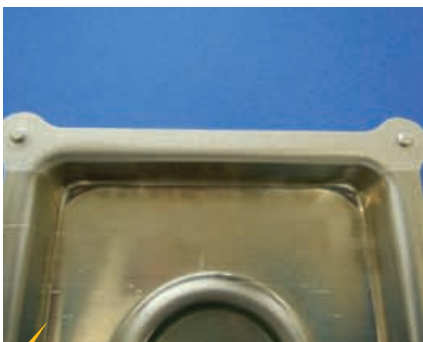
Pre-treated flange of a deep-drawn part prior to adhesive bonding
